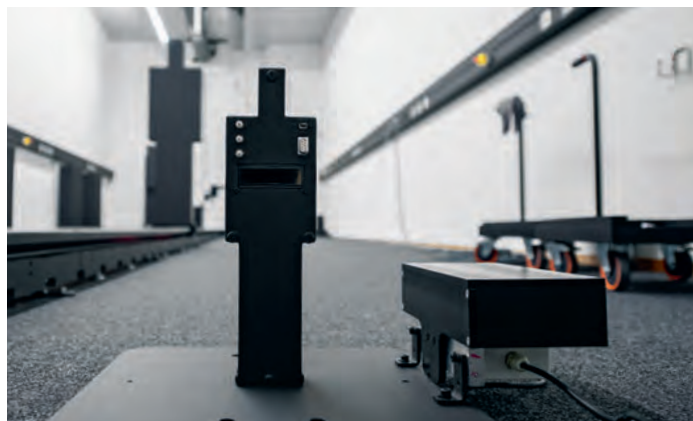
Testing facility for motion and presence sensors for lighting technology.
