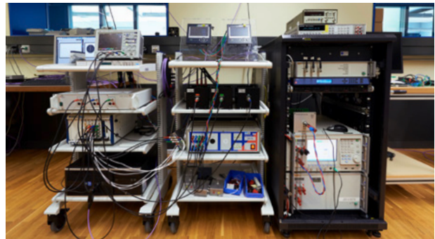
7: More than 150 separate tests must be passed for the certification of a power quality analyser according to the standard IEC 62586-2.
