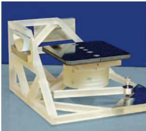
4 Zerodur carrier structure for the three interferometer mirrors which can accommodate also larger samples.
