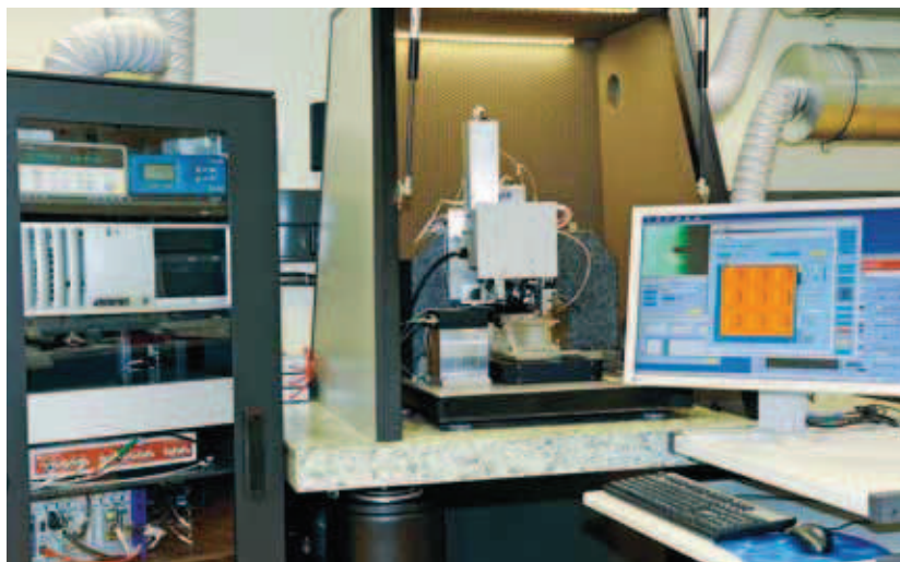
1 3D-AFM set-up in the clean room laboratory of METAS with electronic rack (left), AFM in the opened acoustic box (centre) and control screen (right).
